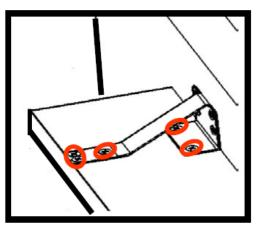
Install Bracket onto Header
